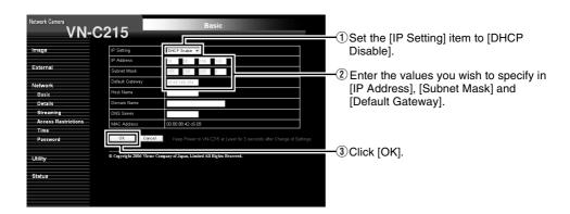
A confirmation screen appears. Press the [OK] button. The VN-C215V4U restarts using the new IP address. It takes about 1 minute for the camera to reboot.
